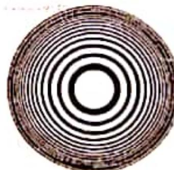
Concentric ring pattern produced by a Fabry-Perot etalon
