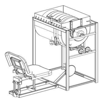
All mechanical parts of the washing machine including operator sitting device should be fabricated and assembled as per the drawing. Details may be available from: Dr. Subhasis Bhaumik (Email: sbhaumik\_besu@yahoo.co.in, subhasis@aero.iiests.ac.in Mobile No. - 9836044278 ). All mechanical parts should be included in the system in assembled condition. The system should have smooth proper surface finish with appropriate coating.
