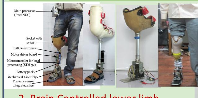
2. Brain Controlled lower limb exoskeleton device for mobility regeneration
