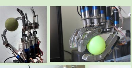
5. Sensor Integrated Multi-Fingered **Dexterous Robot Hand** with Data Glove Interface
