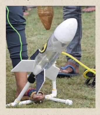
Water Rocket Launch: This hands-on engineering challenge involved building and launching rockets powered by compressed air and water, judged based on height, distance, and creativity of design.
