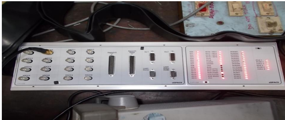
A DSP-based Hardware-in-loop (HIL) system called dSPACE
