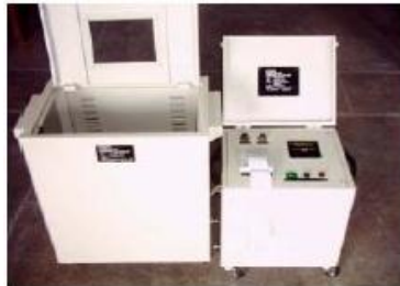
Test Set for measuring Tanδ & BDV
