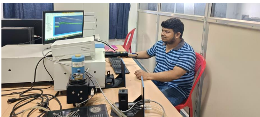
Photon Technology International (PTI) spectrophotometer (Horiba, Delta diode) and multifunctional time-correlated single-photon counting (TCSPC) fluorescence spectrophotometer
